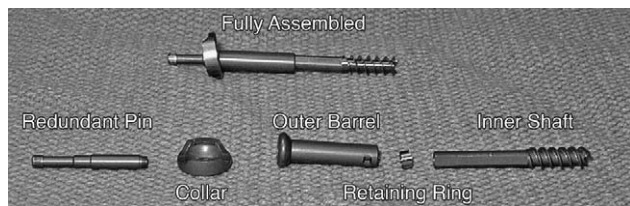
FIGURE 1. Mechanical design of the transfacet fixation device.
