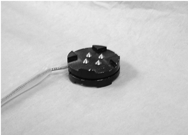
FIGURE 3. Assembled anterior column load cell simulating an interbody cage.
